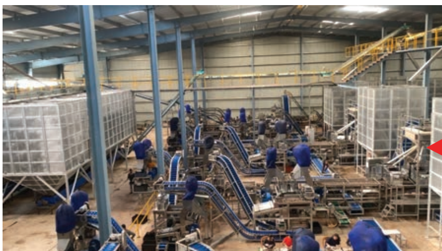
CASHEW PROCESSING PLANT DESIGN 100 TONS RCN/DAY
